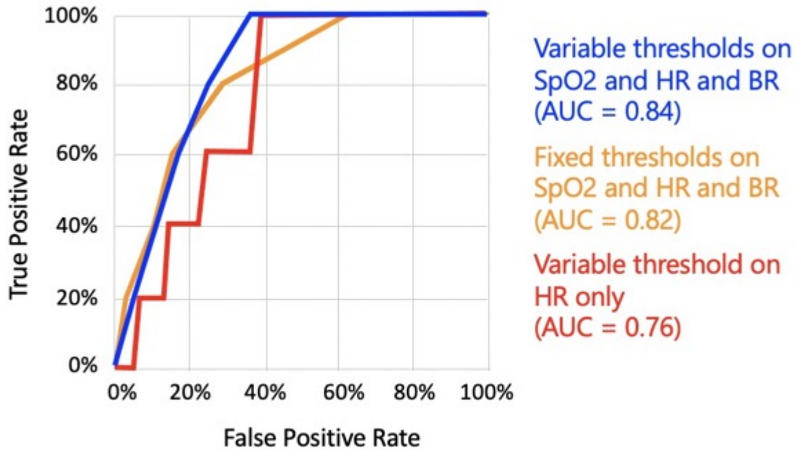
Figure: ROC curve for the early detection of COPD patient at risk of readmission
